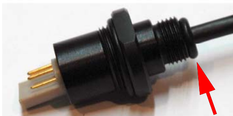
Pic 5: Take care of the right position of the o-ring. (Please note that the contact pins should be more inserted into the plug housing than shown on this picture.)
