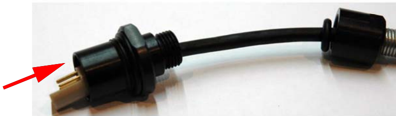
Pic 4: Now press the insert of the plug head carefully into the plug. A bench vice can be helpful. Take care not to damage the contact pins.
