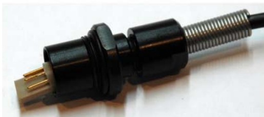
Pic 6: Screw the cable gland to the plug head firmly. Use a flat wrench at the cable holder and a pipe wrench protected with rubber or similar not to damage the plug head.
