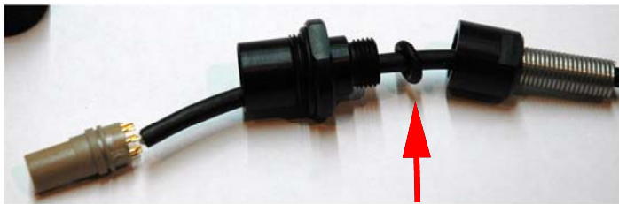
Pic 3: Insert now the cable - please take care of the small o-ring. Solder now the cable ends to the plug.
